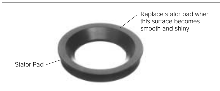
Figure 2. Ultracentrifuge Stator Pad
