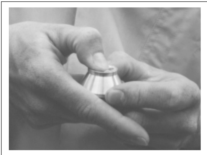
Figure 4. Removing the Rotor Cap. Press in the center of the cap to free an edge.
